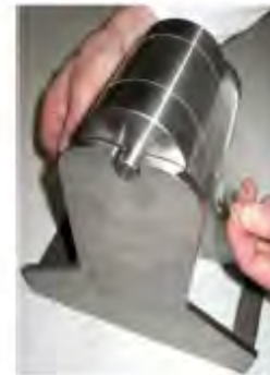
Cylindrical mandrel flexibility (BS EN 435:1994)
